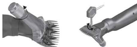
Place the new upper blade in the guide points of the driving carrier; then place a few drops of oil on the ground surfaces. Now push the new lower blade between the loosened screws.
