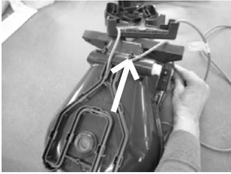
4. Place the heating cable further into the right guide groove and press it into the cable holder. Do not work with pointed tools!
