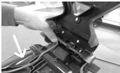
2. Place the heating cable cover together with the heating cable on the rear part of the bowl.
